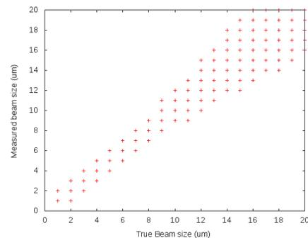
Figure 4: Calculated 1- $\sigma$  statistical resolution contours for 31-element CA with 10  $\mu\text{m}$  elements at the ATF2.
