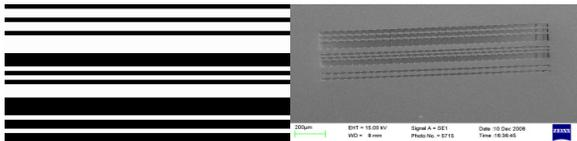
Figure 1: 31-element CA with 10  $\mu\text{m}$  element size. Left: pattern. Right: SEM image from Applied Nanotools. (Adjacent elements of the same type (mask or hole) merge; there are fewer distinct regions than “elements.”)
