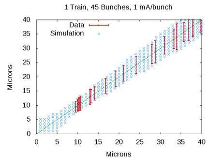
Figure 3: Calculated statistical 1- $\sigma$  resolution contours for CA at CEsrTA for 200 photons/pixel (0.56 mA/bunch). Measured size spreads at 1 mA/bunch are overlaid.
