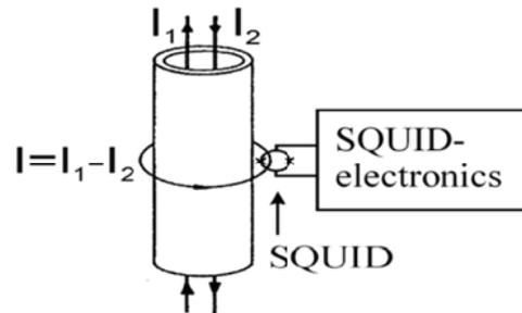
Figure 1: Simplified scheme of an LTS SQUID-based Cryogenic Current Comparator.
