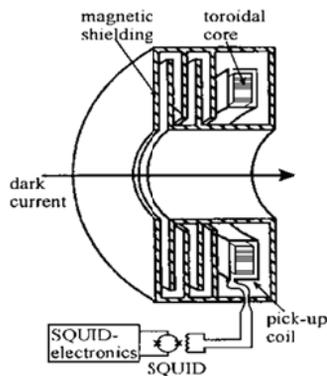
Figure 2: Simplified schematic view of the magnetic shielding, the toroidal pick-up coil, and the SQUID.
