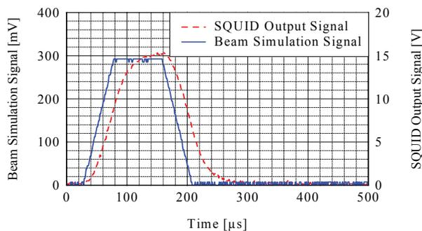
Figure 4: Beam simulation signal (solid line) and output signal of the SQUID based CCC (dotted line).
