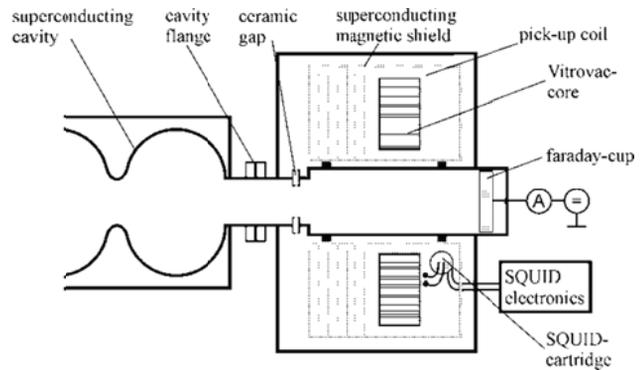
Figure 3: Schematic design of the CCC.
