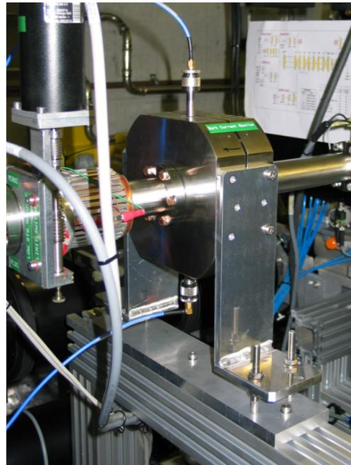
Figure 1: Dark current Monitor at the photo injector test facility.
