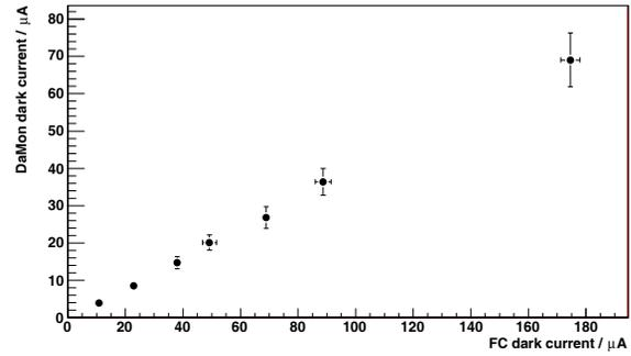
Figure 3: Dark current taken with the DaMon as a function of results with the Faraday Cup.
