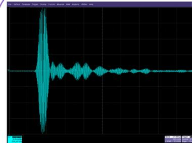
fig 3. Transverse Schottky Signal from the pilot. What we can see after the 1<sup>st</sup> LO
