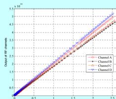
Amplitude response of four channels
