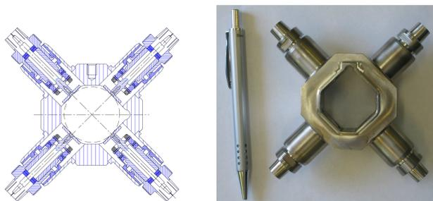
Figure 1: The electrostatic BPM for VEPP-2000 ring.
