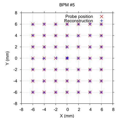
Figure 4: Reconstructed probe position with respect to real one.
