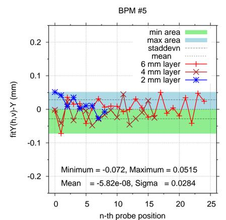
Figure 5: Difference between reconstructed and real probe position.
