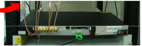
Fig. 7 - Digital Unit based on VHS-ADC board from Lyrtech.
