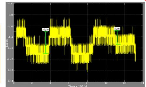
Fig. 8 - Sensitivity of the BPM electronics, measured at the level of 5 μm.
