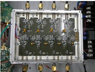
Fig. 4 - AD8310 logarithmic amplifier board.
