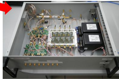
Fig. 3 - AFE unit, including log amp and IQ demodulator boards.
