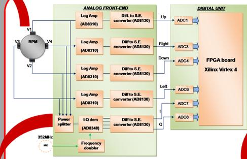
Fig. 1 - ESSB BPM system, with the test-stand and the electronics.
