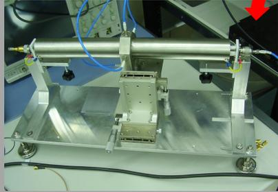
Fig. 2 - ESSB test-stand developed for testing the electronics.
