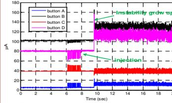
➤ The four blades reading for transverse bunch-by-bunch feedback on/off.
