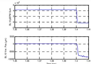
➤ BL 10 Photon BPM post-mortem data. The beam trip occurred at time 1.4 sec.
