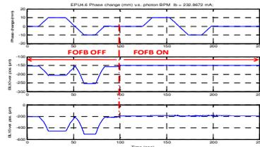
➤ Beamline 10 photon BPM 10Hz reading signal related to the ring BPM.
