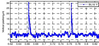
➤ BL10 pBPM vertical position 10kHz readings during injection.
