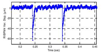
➤ Storage Ring electrical R1BPM4 10kHz readings during injection.
