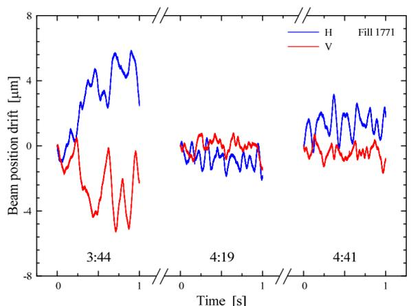
Zoom on the first second of the records from the previous plot. 3:44 – LHC beam at 450 GeV and OFB on, around 4:19 – beam at 3.5 TeV and OFB on, 4:41 – beam at 3.5 TeV and OFB off; ADC acquisition.
