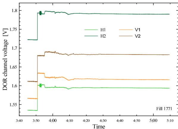
An example of Diode Orbit (DOR) signals acquired with a 6.5-digit laboratory voltmeter at 1 Hz. The DOR front-end was connected to an LHC short-circuited 150 mm stripline BPM of diameter 49 mm. 4 DOR channels were multiplexed with a mechanical relay switch.
