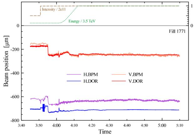
A comparison of beam position calculated from the shown raw DOR signals (theoretical stripline formula) to a standard LHC BPM. Pick-ups of both systems are physically next each other. The presented results are without any prior system calibration.
