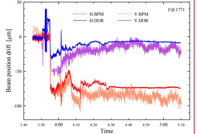
Beam positions as on the plot to the left, but with beam offsets removed at the beginning of the measurement. Around 4:29 the orbit feed-back (OFB) system was turned off.
