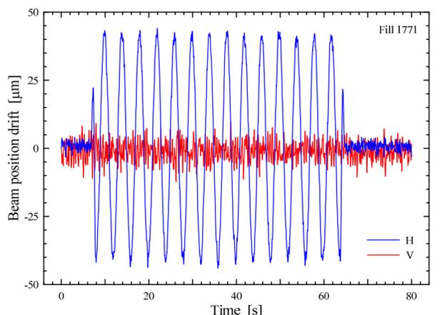
Zoom on beam positions during radial modulation ( $\Delta p/p = 2 \times 10^{-4}$  at 0.25 Hz) seen also on the previous plots around 3:52. The DOR signals were acquired simultaneously (in parallel to the voltmeter acquisition) with 24-bit ADCs at 11.7 kHz.
