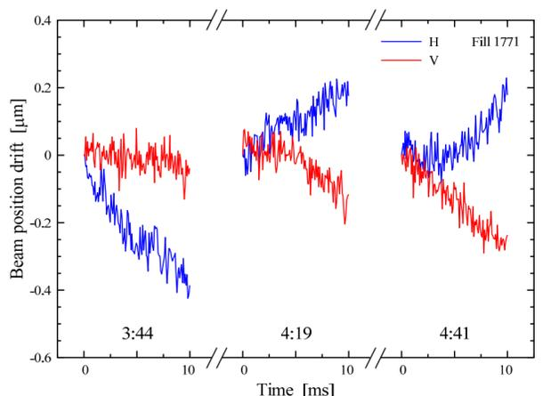
Zoom on first 10 ms (some 112 LHC revolutions) of the records from the previous plot. 3:44 – LHC beam at 450 GeV and OFB on, around 4:19 – beam at 3.5 TeV and OFB on, 4:41 – beam at 3.5 TeV and OFB off; ADC acquisition.
