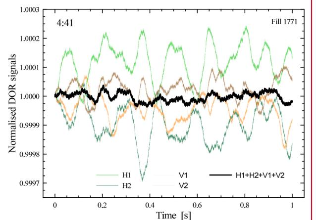
Zoom on the first second of raw DOR signals and their sum, record of 4:41, OFB off, ADC acquisition at 11.7 kHz.
