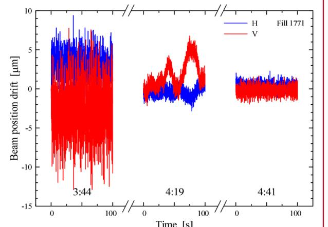
Zoom on 100-second DOR signal records around 3:44 – LHC beam at 450 GeV and OFB on, around 4:19 – beam at 3.5 TeV and OFB on, as well as around 4:41 – beam at 3.5 TeV and OFB off; ADC acquisition.
