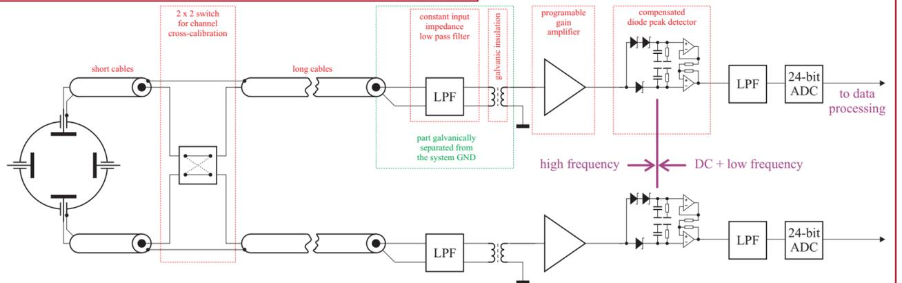
One plane of the Diode Orbit (DOR) measurement system consists of two symmetrical channels converting fast beam signals from the opposing electrodes of a position pick-up into slowly varying DC signals. The multiplexer is foreseen for cross-calibration of each channel pair.
