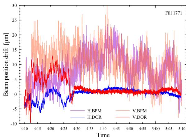
Last hour of measurements presented on the previous plot with beam offsets forced to zero at the end.
