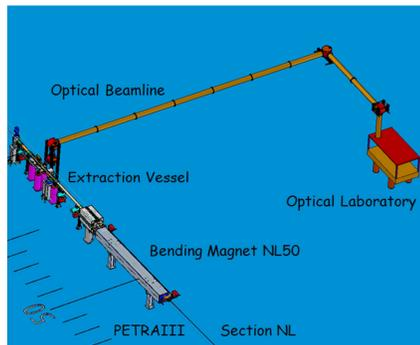
The measurement of the bunch length of the PETRAIII storage ring is based on the analysis of visible synchrotron radiation from a bending magnet [1]. The main parameters, characterising the storage ring and the bending magnet light source are given below:
