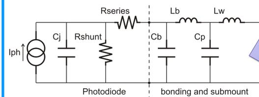
Photodiode equivalent circuit:
