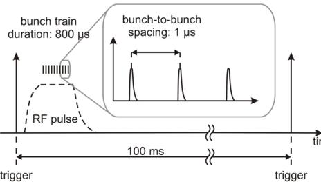
Pulse mode timing scheme for FLASH operation.
