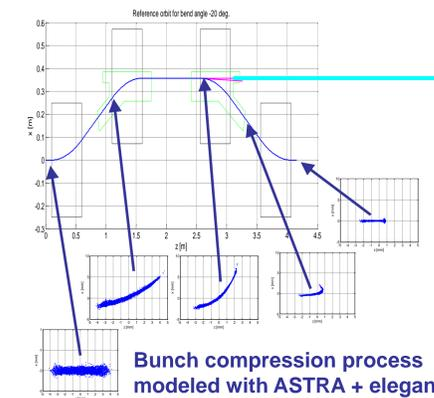
Horizontal beam position  $\Delta x$  in the dispersive section of bunch compressor is related to the beam energy  $\Delta E/E$  by  $\Delta x = R_{16} * \Delta E/E$  with  $R_{16} \sim 300-360$  mm, where  $R_{16}$  is the horizontal dispersion
