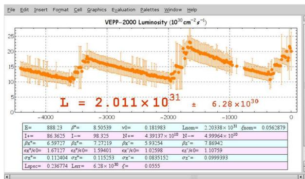
Figure 4: Online Luminosity calculations based on beam sizes measurements along the ring.
