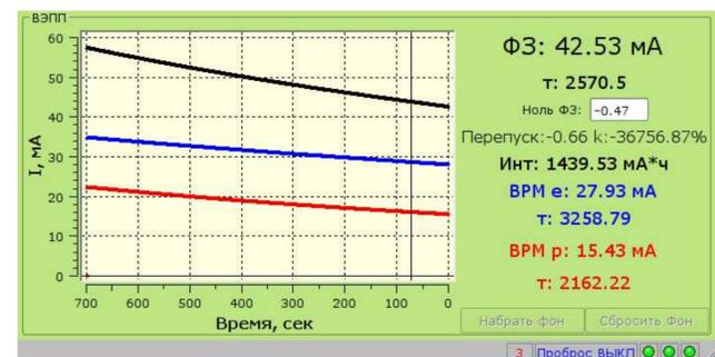
Figure 6: Beam currents and life time monitor.
