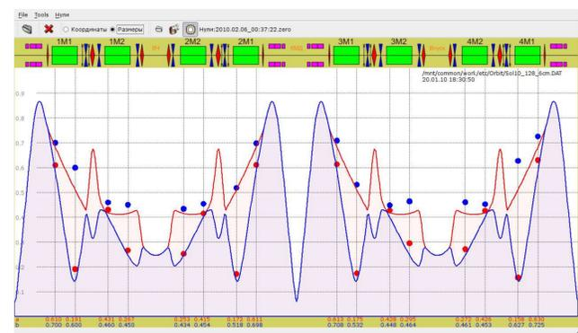
Figure 5: Beam sizes along the ring vs. lattice model.
