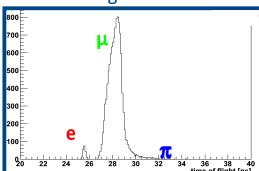
**Low momentum spread:** beam for calibration of the detectors:
