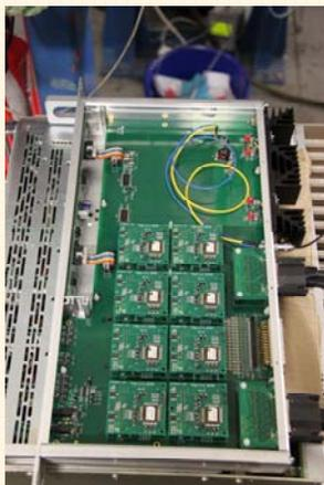
Prototype board with 8 CFC-ASICs
