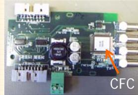
CFC-test board with I/O-drivers
