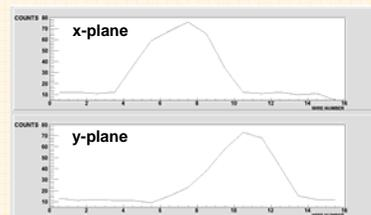
Original SEM-grid image of a  $^{124}\text{Xe}^{21+}$  ion beam @ 4.773 MeV/u. The beam current is around 6μA and has a pulse length of 100μs. The horizontal beam profile (x-plane, 16-wire grid) as well as the vertical beam profile (y-plane, also equipped with 16 wires) are shown. This kind of images can prepare also the existing old hard- and software. An example with the new readout electronics is presented beneath.
