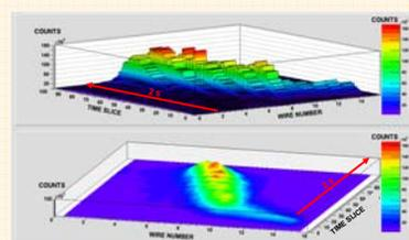
Original MWPC images of an  $^{40}\text{Ar}^{18+}$  ion beam @ 300MeV/u. Both figures show the vertical and time-dependent beam profiles from the first half of the MWPC x-plane (wire 1 to 16). The beam pulse length is around 1.8 s and each time slice length is 20ms. The ion beam was mismatched knowingly to present the new feature of the prototype. Both diagrams present the same beam profile, but in a different graphical representation.
