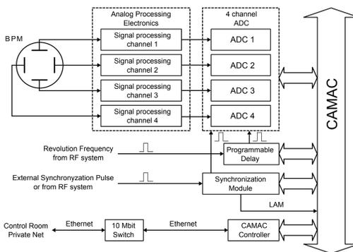
Figure 2: Structure of VEPP-2000 electronics.
