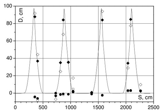
Figure 5: Dispersion function. Point near picks maximums is the BPM measurements.
