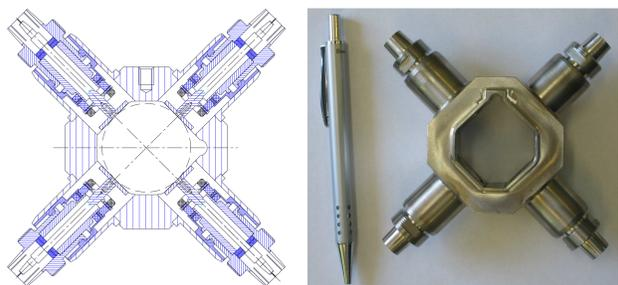
Figure 1: The beam position monitor for VEPP-2000 ring.
