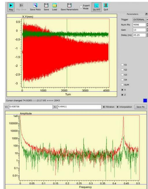
Figure 3: Beam oscillation after external kick during 4000 turns and their betatron spectra.
