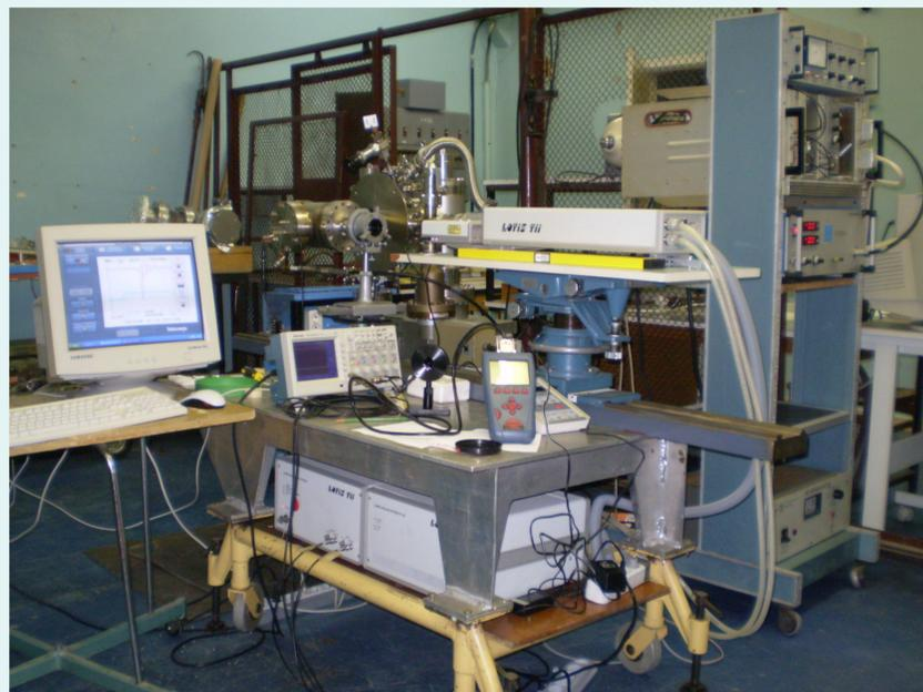
Cathode investigations were done at a stand with a monopulse YAG:Nd<sup>3+</sup> laser. Generated radiation had wavelength of 266 nm, pulse length of 15 ns and maximum energy of 15 mJ.
