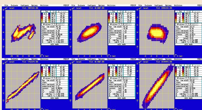
High current  $^{40}\text{Ar}^{+}$  beam emittances in front of (left, **I**) and behind (**i**) the HSI RFQ with original (middle) and new electrodes (right). The emittances reflect the larger acceptance of the new electrodes.
