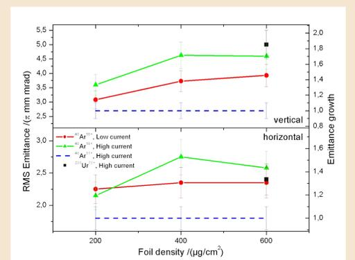
Stripping of different ion beams was studied for 3 foil densities at **IV**, **VI** and **VII**.
