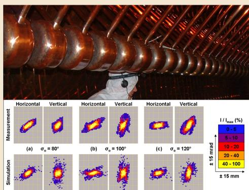
Emittance growth in the periodic Alvarez structure (top left) was investigated (**III**, **IV** and **ii**). At high beam currents resonant growth is excited at transverse phase advance  $90^\circ$  (left bottom & middle). Simulation and experimental data were benchmarked (middle & left).
