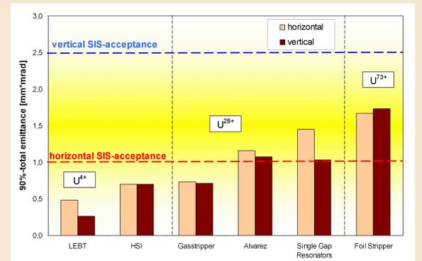
Emittance growth along the UNILAC can be monitored by the permanent devices **I-VIII**; matching the main DTL and foil stripping are the main sources.
