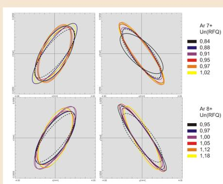
Output beam emittances of the new HLI RFQ at **iv** for  $^{40}\text{Ar}^{7+/8+}$  for different normalized rf amplitudes; dashed: original design.
