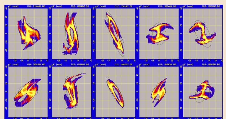
Transverse emittances measured at **iii** reveal the rich phase space structure of an ECRIS  $^{40}\text{Ar}$  beam, resulting in manifold emittance figures for different beamline (matching to RFQ) and source settings.
