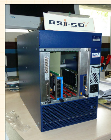
μTCA crate test installation
