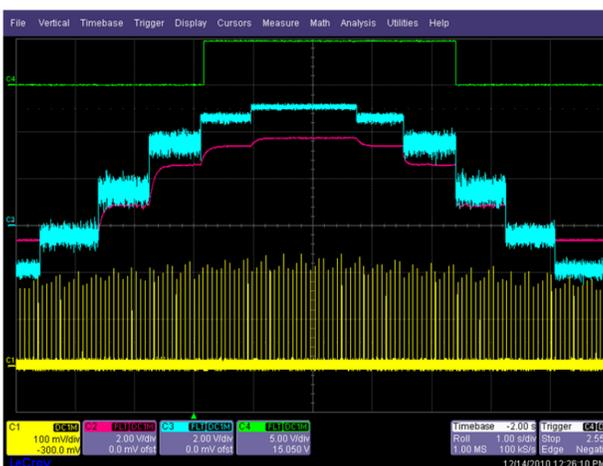
Threshold measurement with the effect of the asymmetric low pass filter.
