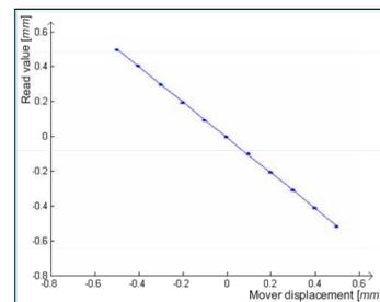
Result of the calibration, tolerance: 10%
