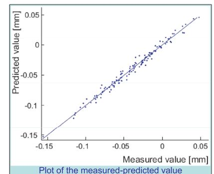
This resolution method compares the reading of the electron beam offset measured with the BPM of interest ('m'), with the predicted value by all the other BPMs [3]. The data is acquired in real time mode, in presence of beam jitter.
