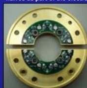
The main benefits of IPU's: position and current intensity measurements in the same device, less perturbed from the high losses in linacs, high output dynamic range for beam currents in the range of interest, broad bandwidth for pulsed beams and short total length.
