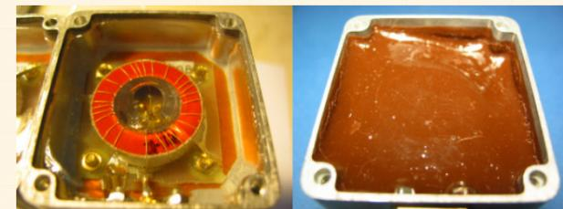
Figure 7: Materials whose structure was destroyed during the thermal cycling: Stycast 1266 A/B (left), Araldite CW 299 (right) and Stycast 2850 FT (not shown).
