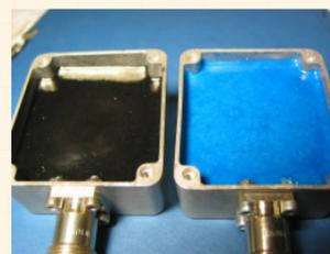
Figure 6: Samples that survived cryogenic tests: Stycast 2850 KT (left) and Stycast 2850 KT (right).
