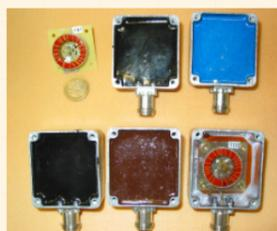
Figure 5: Matching transformers non-encapsulated and encapsulated in epoxy (from left top to down bottom). The order is the same as in Table 1.
