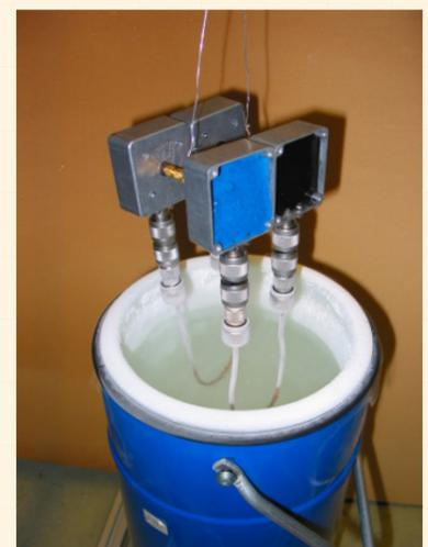
Figure 8: Cryogenic test of encapsulation samples. Extension out of semi-rigid cables used to slow down the cooling. Otherwise shock cooling would generate additional stress in epoxy and toroid material.
