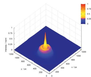
Fig. 8: Beam luminosity density reconstruction slice. Ring structures become visible.
