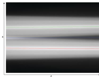
Fig. 3: Plot of beam imaged at 0° (upper) and 180° (lower) beam axes (green, red) and corresponding correction axis (blue) are displayed as an overlay.
