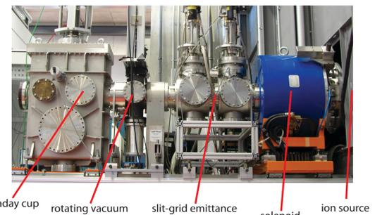
In a first tomographic measurement we took 181 images from 0° to 180°. The ion beam was focused with 0.21 T resulting in 13 mm beam diameter at the rotating vacuum chamber.
