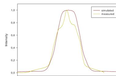
Fig. 7: Beam profile taken at 0° in the rotating vacuum chamber and simulated profile integrated over z. Asymmetric drop-off from maximum to beam boundaries in measured profile.
