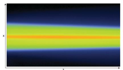
Fig. 6: Beam profiles taken at 0° in the rotating vacuum chamber. Image post processed with background subtraction and vignetting correction.
