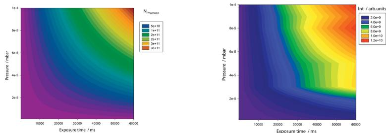
Fig. 1: Theoretical plot of photon production dependent on pressure and time.
