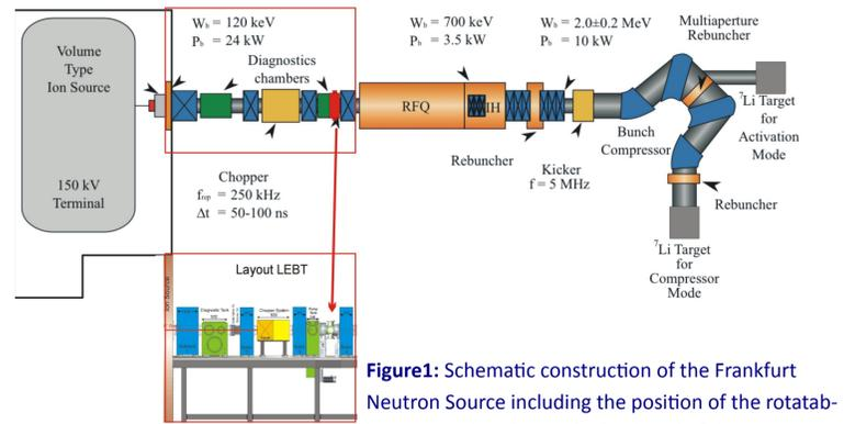
Figure 1: Schematic construction of the Frankfurt Neutron Source including the position of the rotatable vacuum chamber in the back end of the LEBT.
