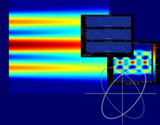
**A** non-interceptive optical diagnostic system on the basis of beam tomography, was developed for the planned Frankfurt Neutron Source (FRANZ). The proton driver linac of FRANZ will provide energies up to 2.0 MeV. The measurement device will non-interceptively derive required beam parameters at the end of the LEBT at beam energies of 120 keV and a current of 200 mA. On a narrow space of 351.2 mm length a rotatable tomography tank will perform a multi-turn tomography with a high and
