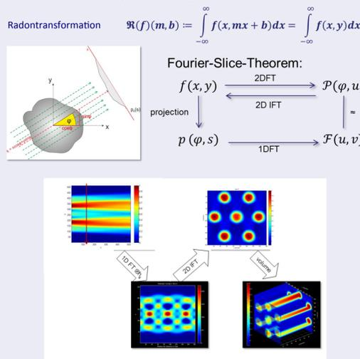
Figure 6: example of position space tomography on a simulated 7-beamlet beam
