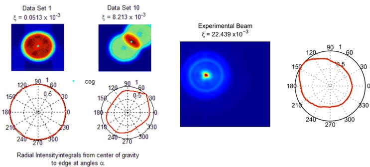
Figure 3: The symmetry analysis used to compare different beams. On the left, two examples of the 10 data sets are compared. The left one is nearly radial symmetric, the right one is axis symmetric. On the right hand side a measured beam is analyzed.
