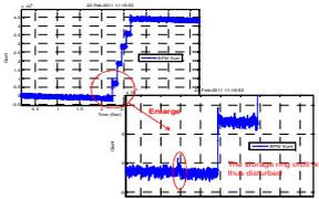
➢R1BPM3 10 kHz sum readout. The red circle of the below picture remarks that booster has no current but pulse magnet still fired caused the orbit disturbed.
