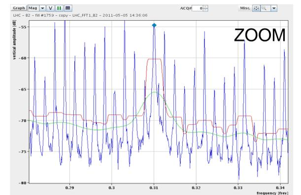
"Forest" of  $Q_s$  lines due to longitudinal bunch phase and shape oscillations (machine development)
