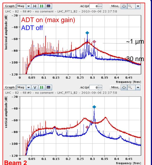
Higher transverse bunch-by-bunch FB (ADT) gain implies also more measurement noise propagated onto beam  $\rightarrow$  nullifies the higher BBQ sensitivity
