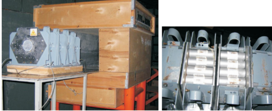
E+T: 4 sections lead target in natural uranium blanket
