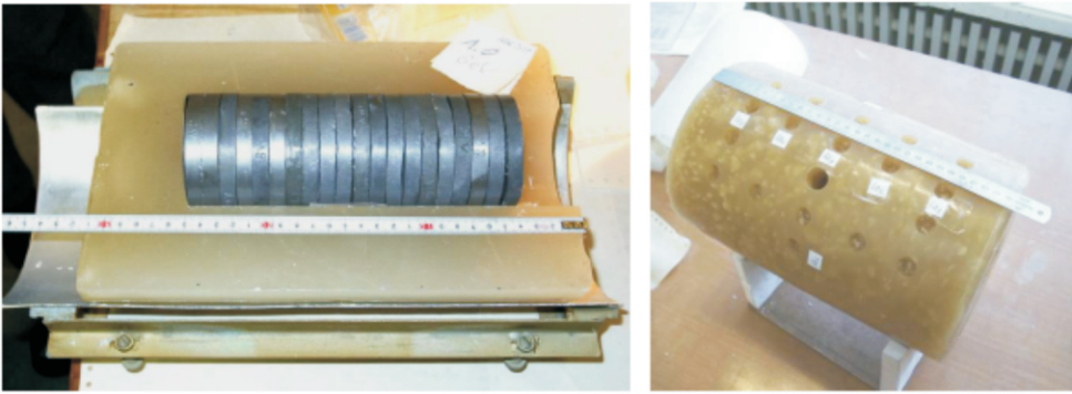
Gamma-2: lead target in paraffin
