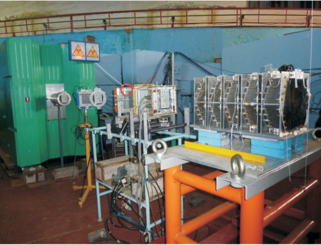
Quinta: 5 sections natural uranium target
