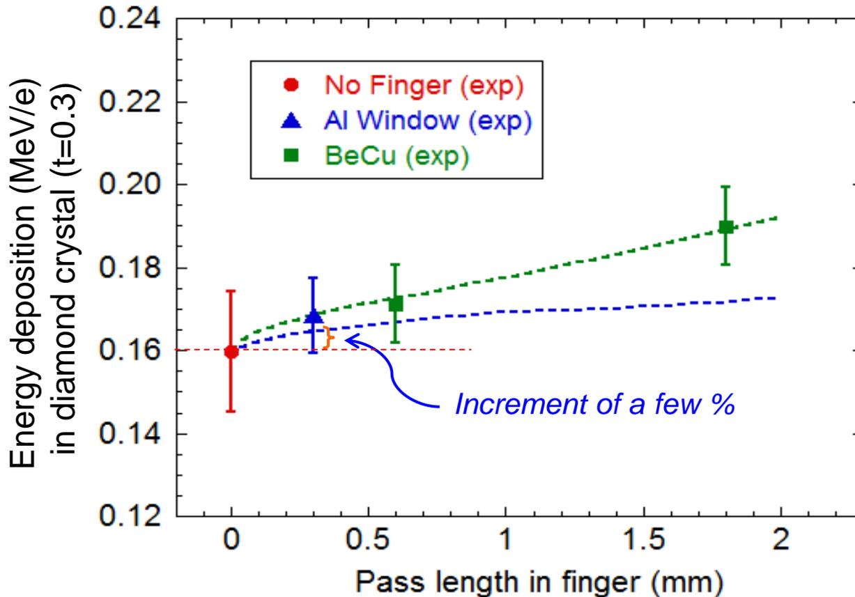
Dashed lines are simulation results by Monte Carlo simulation code: EGS5.
