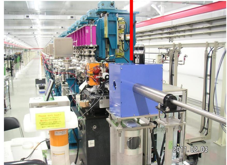
The Halo Monitor equipped with RF fingers (type 2).
