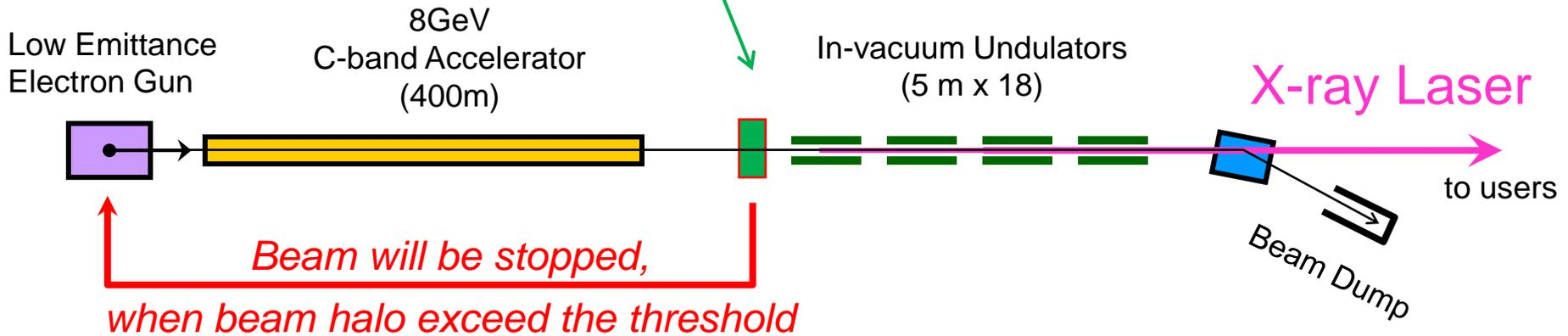
*If the undulator magnets are irradiated with beam halo, the magnets are **fatally demagnetized**.*
