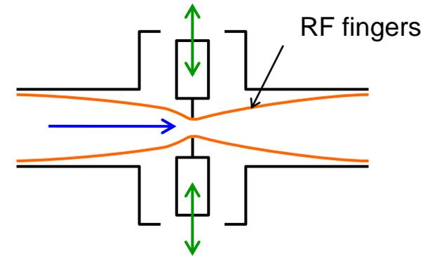
In the configuration of **type 1**, the active areas of the diamond detectors project from between RF fingers.
