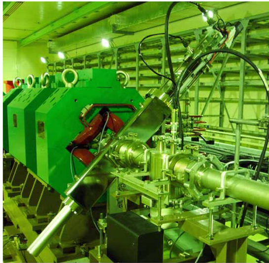
Wire scanner (LINAC)
