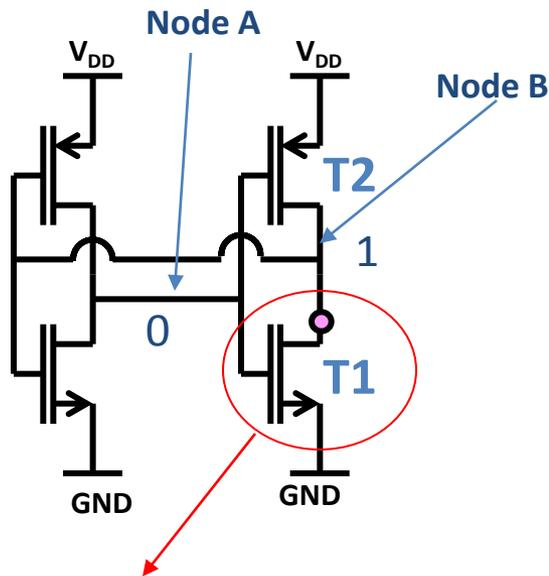
Charge collected at the drain of NMOS T1 tends to lower the potential of the node B to gnd. PMOS T2 provides current from Vdd to compensate, but has a limited current capability. If the collected charge is large enough, the voltage of node B drops below  $V_{dd}/2$
