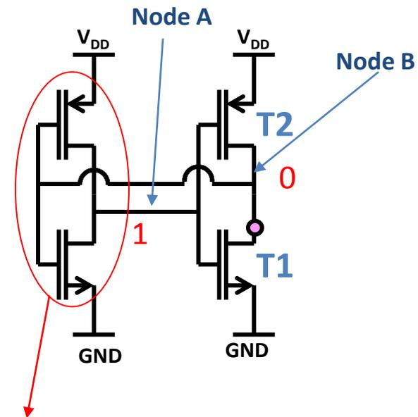
When node B drops below  $V_{dd}/2$ , the other inverter in the SRAM cell changes its output (node A) to logic 1. This opens T2 and closes T1, latching the wrong data in the memory cell.
