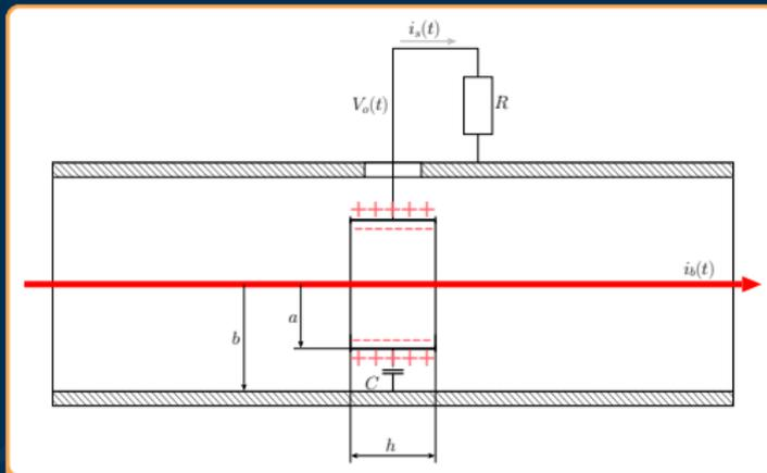
Principle of capacitive pick-up
