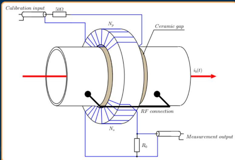
Fast Beam Current Transformer
