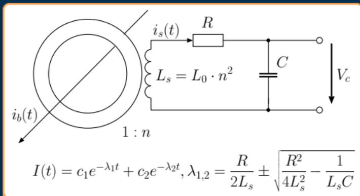
FBCT equivalent lumped circuit
