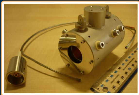
SE deflection using electrostatic shielding
