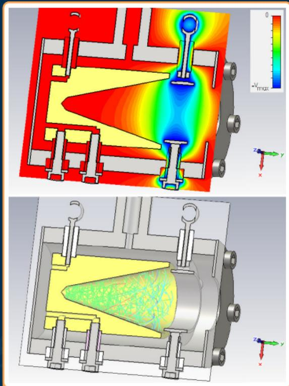
SE deflection using electrostatic shielding
