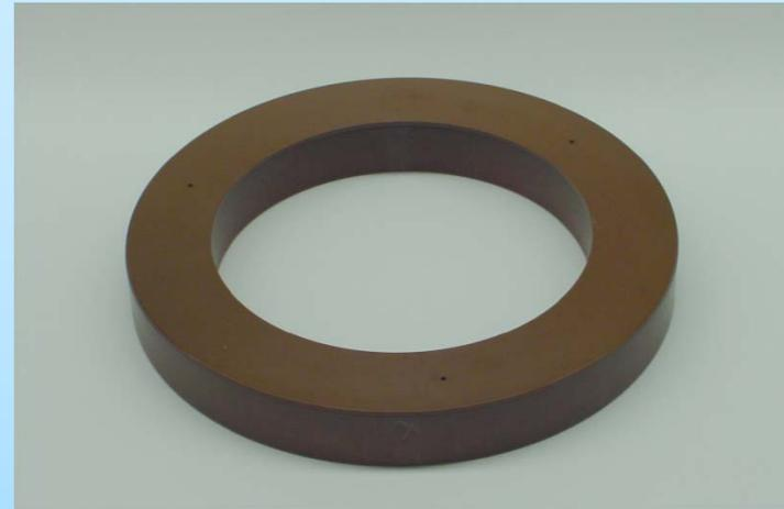
Toroidal core (VITROVAC 6025-F) housed in a VESPEL insulator.
