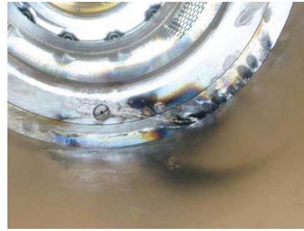
Figure 9: Damage caused by sparking between ground shield, that protects the 40kV insulator, and the high voltage surface. The ground shield is removed here, exposing the 40kV insulator.
