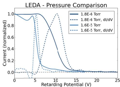
Figure 7: Measured beam potential for two different Ar pressures in the beam line. Beam current = 6.2 mA. The spectrum on the left was taken at the higher pressure. The neutralizations were about 64% for the lower pressure and 89% for the higher pressure.
