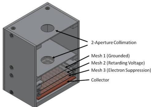
Figure 2: Cut isometric view of the RFA.
