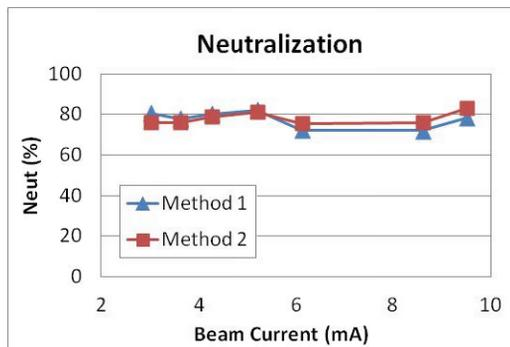
Figure 6: Neutralization level vs. beam current. The pressure in the beam line was  $4.2E-6$  Torr. For a description of methods 1&2 cf. text.
