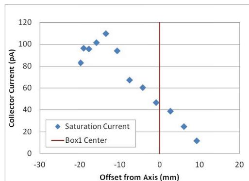
Figure 9: SuSI: RFA saturation current as a function of offset from the chamber center.
