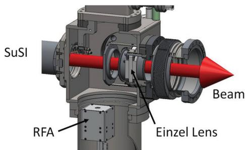
Figure 1: RFA in SuSI LEBT – diagnostic box 1. The Einzel Lens was turned off during measurements.
