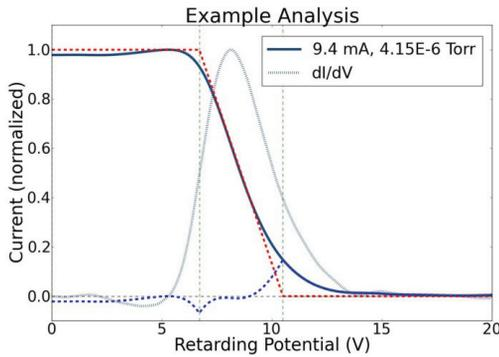
Figure 3: LEDA, Example Analysis of a LEDA ion source neutralization spectrum. The solid blue line is the normalized spectrum, the dotted line is  $dI/dV$  and the dashed red lines are the fit according to method 2. Method 1 would use the base width of  $dI/dV$  as  $\Delta\phi$ .  $\Delta\phi_{\text{meth.1}} = 4.6$  V,  $\Delta\phi_{\text{meth.2}} = 3.8$  V and  $f_{c1} = 78.4\%$ ;  $f_{c2} = 83.0\%$ .
