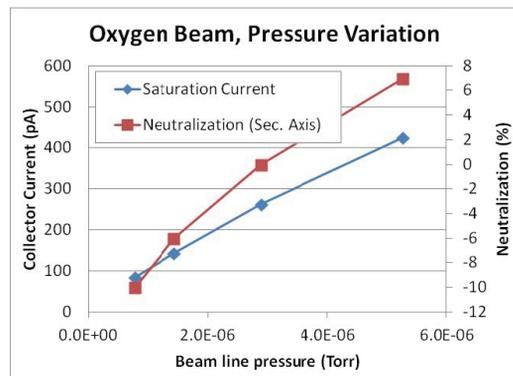
Figure 8: SuSI, oxygen beam, pressure variation. total beam current  $\sim 2$  mA.
