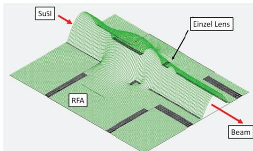
Figure 10: Potential map of beam space-charge potential. The cut is made vertically at the beam-line center.
