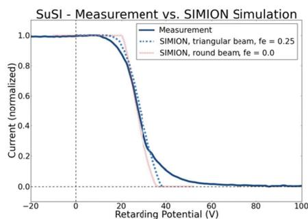
Figure 11: Comparison of a spectrum obtained with SuSI and SIMION simulations. Solid line: Measurement. Dashed line: Assuming triangular beam and 25% neutralization. Dotted line: Assuming round beam without neutralization. Both simulations used the same parameters otherwise.
