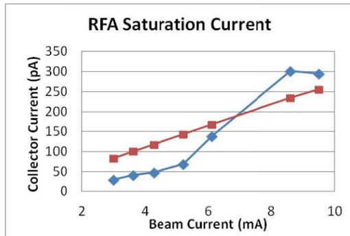
Figure 5: Blue diamonds: RFA saturation current on collector, red squares: Calculation with continuity equation using  $T = 0.1$  (cf. Text).
