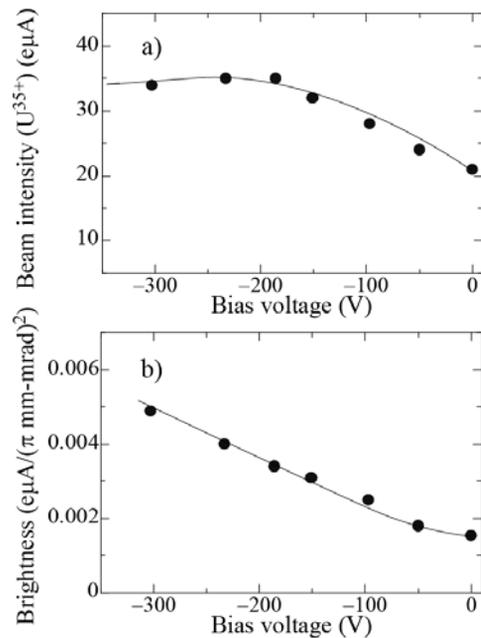
Figure 7: a) Beam intensity and b) brightness of  $\text{U}^{35+}$  ion beam as a function of disc voltage.
