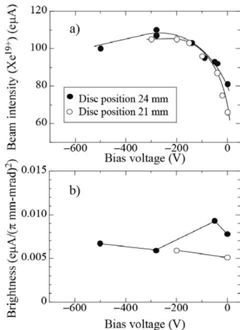
Figure 6: a) Beam intensity and b) brightness of  $\text{Xe}^{19+}$  ion beams as a function of disc voltage.
