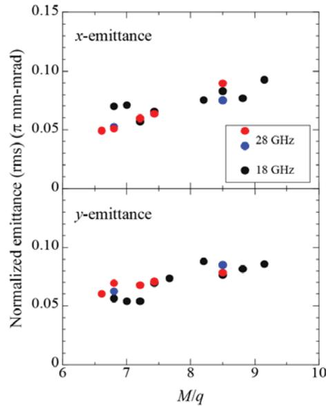
Figure 4: 4 rms emittance for highly charged U ion beams for 28 and 18 GHz microwaves (red and blue circles indicate the value obtained for 28 GHz microwaves for different measurement runs).
