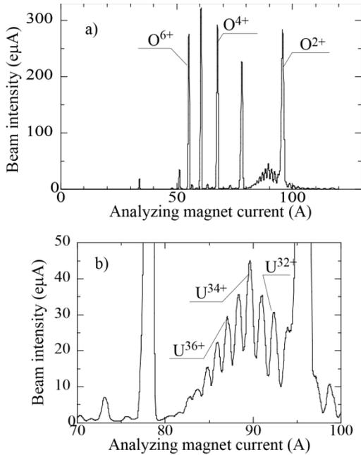
Figure 2: Charge state distributions for O and U ion beams.
