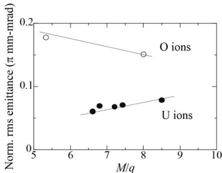
Figure 3: Normalized rms  $x$ -emittance for O and U ion beams.
