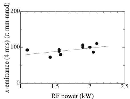
Figure 5: 4 rms  $x$ -emittance for  $U^{35+}$  ion beams as a function of RF power.
