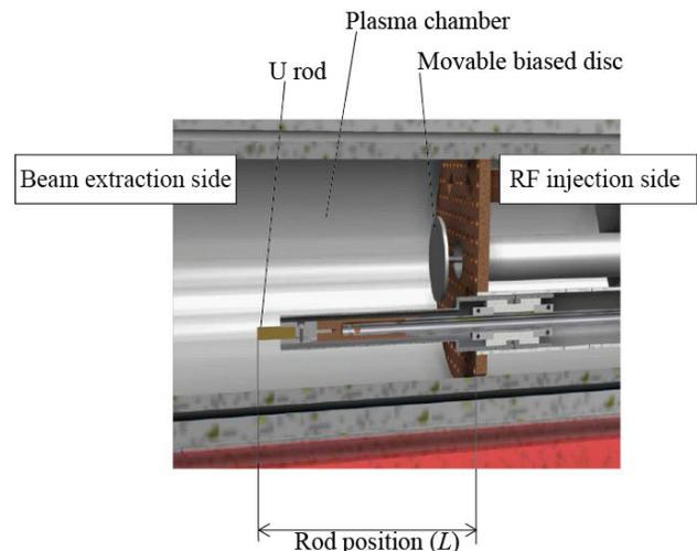
Figure 1: Schematic illustration of the RF injection side of the plasma chamber.
