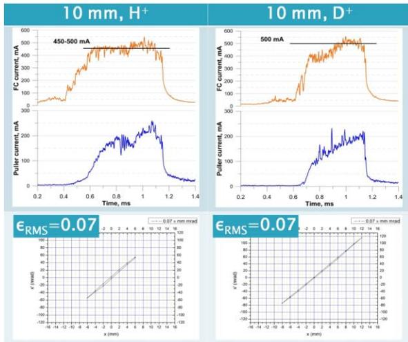
Figure 2: Faraday cup (FC) and puller current oscillograms for H<sup>+</sup> and D<sup>+</sup> beams and corresponding emittance diagrams obtained with 45 kV extraction voltage.
