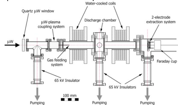
Figure 1: SMIS 37 experimental setup.
