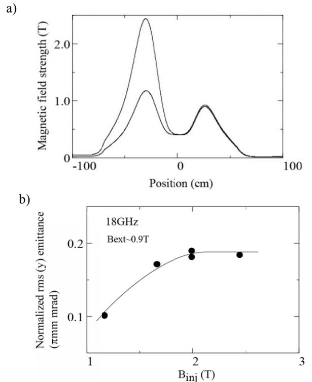
Figure 12: a) Magnetic field distribution for studying the effect of  $B_{inj}$ , b) Normalized rms emittance as a function of  $B_{ext}$ .
