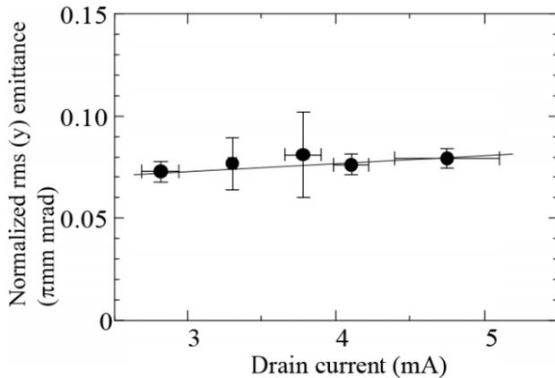
Figure 2: Normalized rms emittance as a function of drain current.
