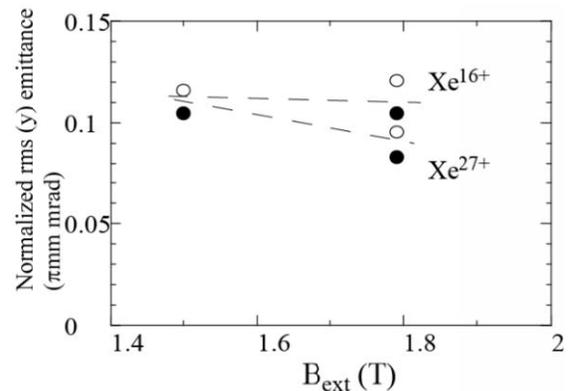
Figure 14: Normalized rms y-emittance for highly charged Xe ions as a function of  $B_{ext}$ .
