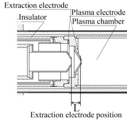
Figure 3: Schematic of the beam extraction side.
