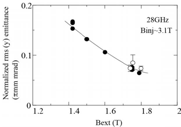
Figure 6: Normalized rms y-emittance as a function of  $B_{\text{ext}}$ .
