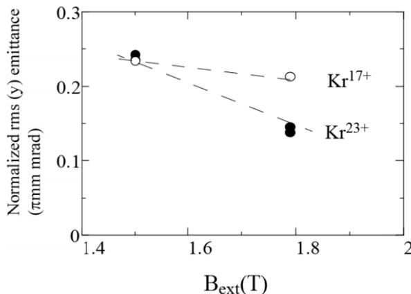
Figure 13: Normalized rms y-emittance for highly charged Kr ions as a function of  $B_{ext}$ .
