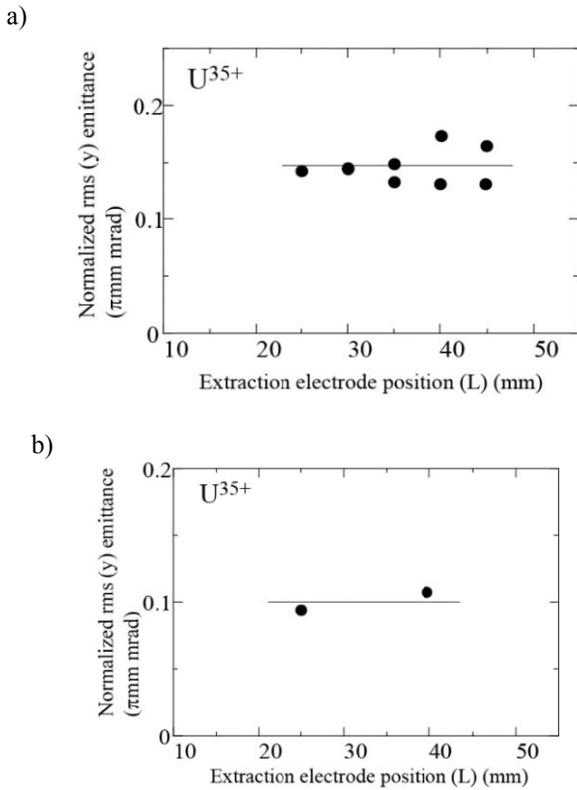
Figure 10: Normalized rms y-emittance as a function of extraction electrode position. a)  $B_{inj} \sim 3.1$  T,  $B_{min} \sim 0.65$  T,  $B_{ext} \sim 1.45$  T, and  $B_r \sim 1.8$  T; b)  $B_{inj} \sim 1.6$  T,  $B_{min} \sim 0.65$  T,  $B_{ext} \sim 1.45$  T, and  $B_r \sim 1.8$  T.
