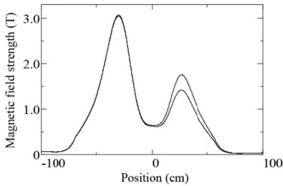
Figure 5: Magnetic field distribution for the  $B_{\text{ext}}$  effect with 28-GHz microwaves.
