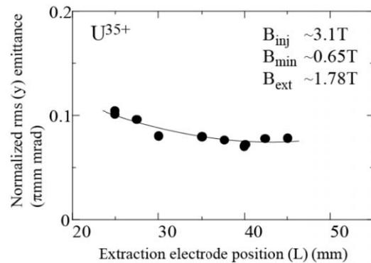
Figure 4: Rms emittance as a function of extraction electrode position ( $L$ ).
