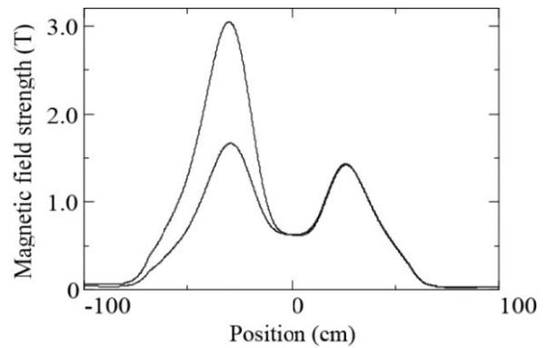
Figure 7: Magnetic field distribution for the  $B_{\text{inj}}$  effect with 28-GHz microwaves.
