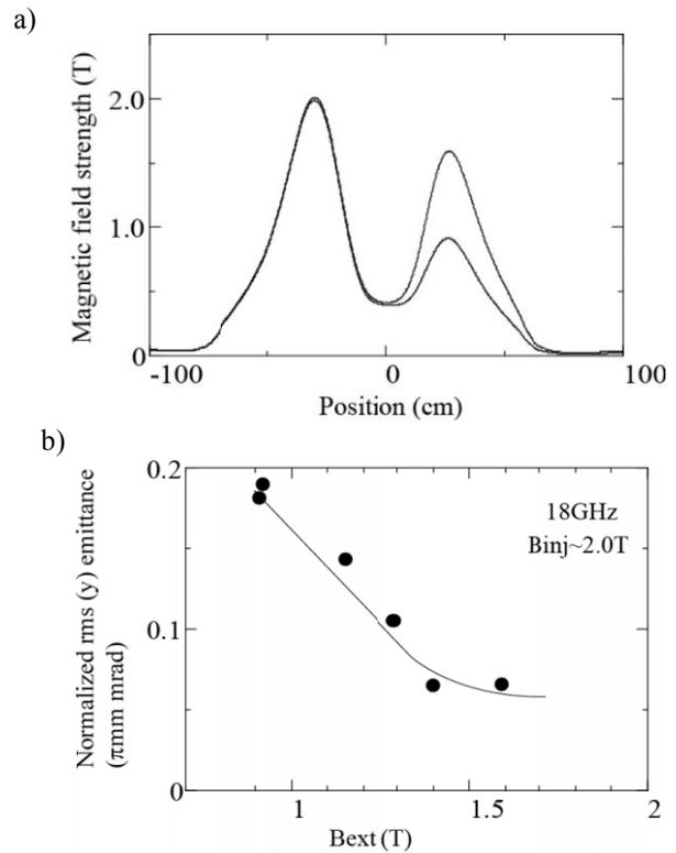
Figure 11: a) Magnetic field distribution for studying the effect of  $B_{ext}$ , b) Rms emittance as a function of extraction electrode position.
