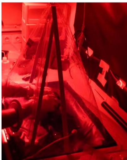
Figure 1: a portable glow bag for the sample manipulation.
