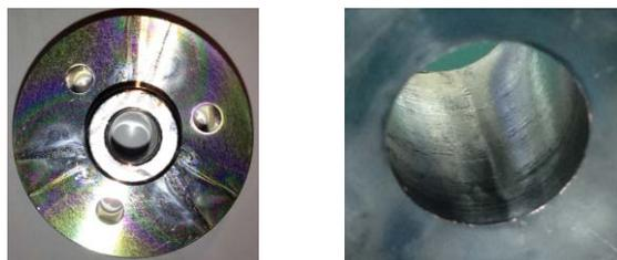
Figure 5: Used plasma electrode (left) and ion deposition in the tube after a year's operation in the ECR ion source for  $C^{4+}$  (right).
