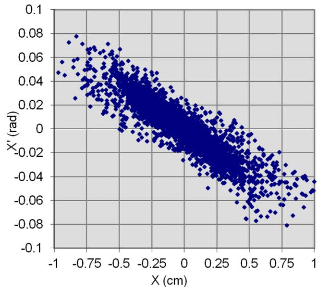
Figure 6: The calculated output phase space in the y plane of the  $\text{U}^{40+}$  charge state extracted from the 56 GHz ECR and transmitted through the RFQ.
