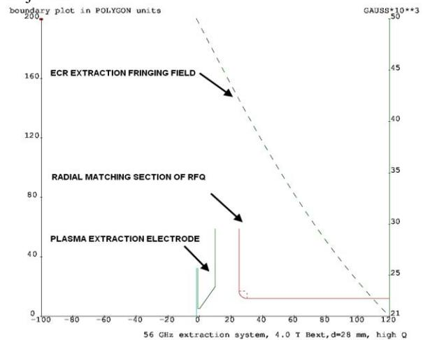
Figure 1: Geometry of the problem simulated with IGUN.
