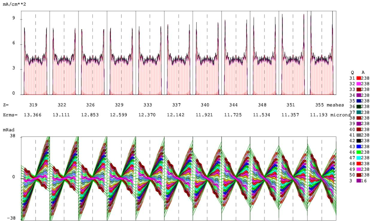
Figure 3: Current densities and RMS emittances of the  $U^{40+}$  ions, other  $U^+$  charge states, and oxygen mixing gas components inside the RFQ matching section.
