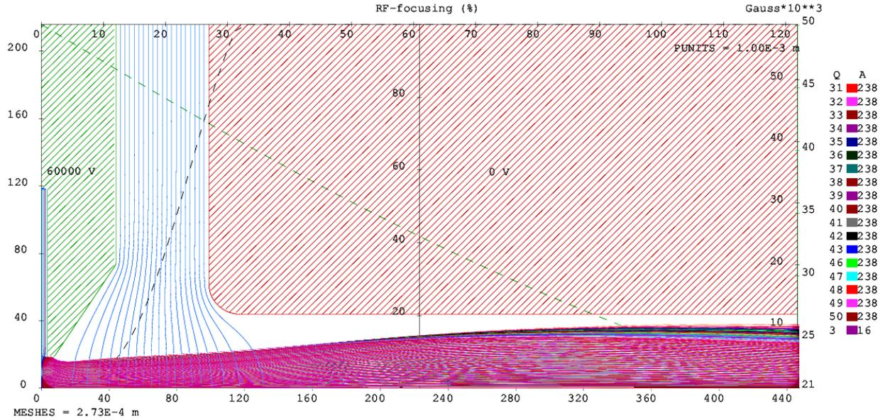
Figure 2: Optimized design for transporting a total current of 12 mA (from 56 GHz ECR source), consisting of  $U^{40+}$ , other  $U^+$  charge states, and oxygen mixing gas ions directly into an RFQ.
