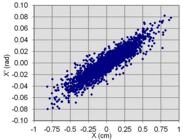
Figure 5: The calculated output phase space in the x plane of the  $\text{U}^{40+}$  charge state extracted from the 56 GHz ECR and transmitted through the RFQ.
