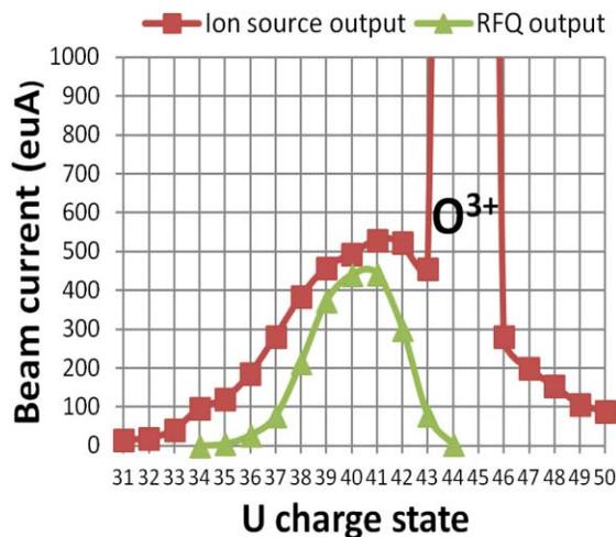
Figure 4: The scaled  $\text{U}^+$  charge states extracted from the 56 GHz ECR and the calculated charge states transmitted through the RFQ.
