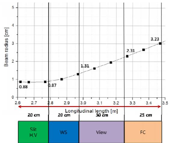
Figure 4: The beam radii in the diagnostic chamber
