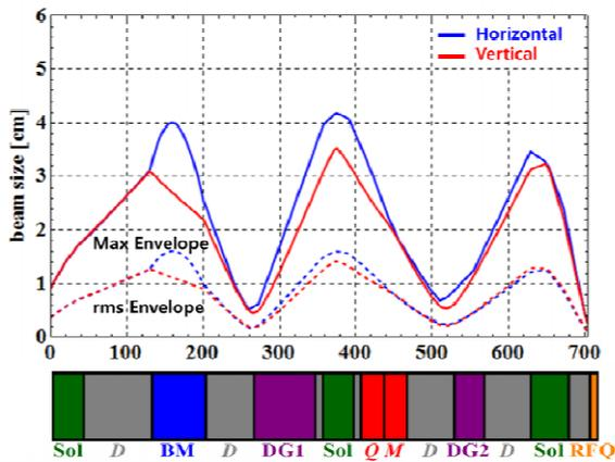
Figure 3: The results of the beam optics simulation.
