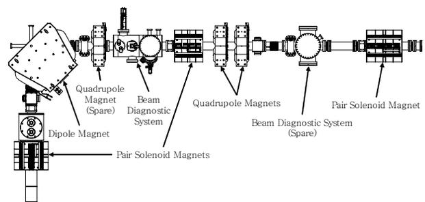
Figure 2: Schematic diagram of the LEBT system.
