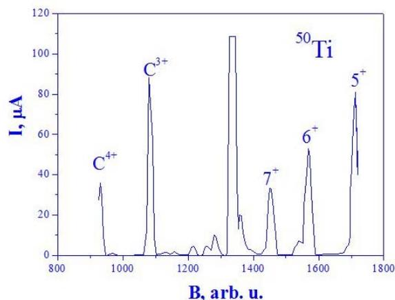
Figure 5:  $^{50}Ti$  ion spectrum, produced by MIVOC method from the ECR4M source at microwave power of 30 W.
