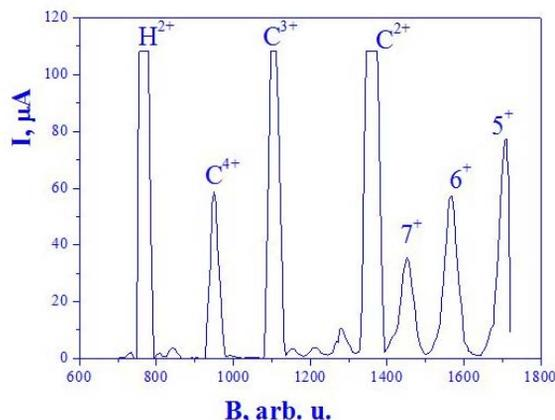
Figure 3: Ti ion spectrum, produced by MIVOC method from the ECR4M source at microwave power of 20 W.
