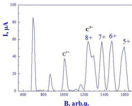
Figure 2: Ti ion spectrum produced by MIVOC method from the DECRIS-4 ion source.
