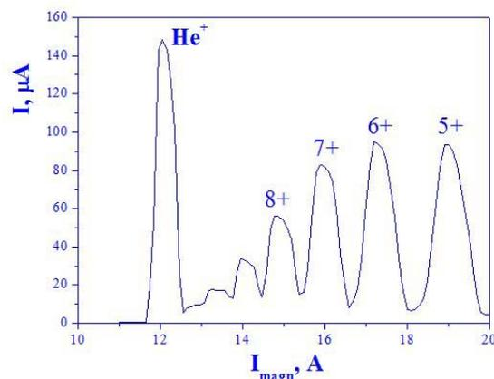
Figure 1: Ti ion spectrum produced by rod insertion from the DECRIS-2 ion source.
