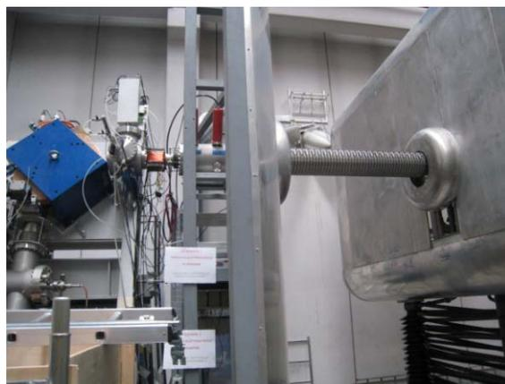
Figure 3: 400 kV high voltage platform, accelerating tube, electrostatic quadrupoles and PM1.
