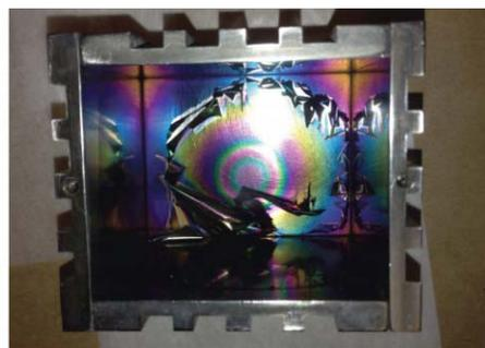
Figure 2: Ytterbium metal deposited on the collector plates.
