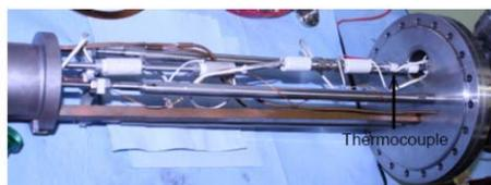
Figure 7: A photograph of the transfer line to transmit cadmium vapor through the ARTEMIS injection assembly with minimal losses. Heating elements are visible (white boxes) and an arrow points to our thermocouple (on right).
