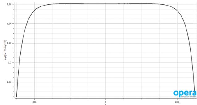
Figure 5: Radial component along z at the inner wall of the AISHa plasma chamber (radius=46 mm).
