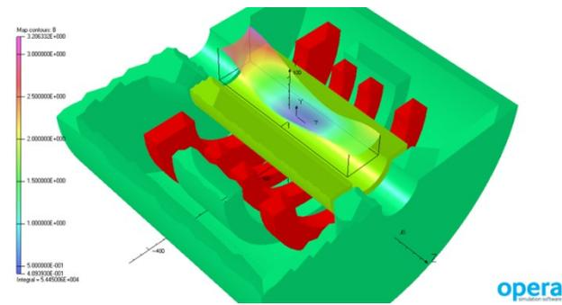
Figure 4: A 3D view of the entire magnetic system.
