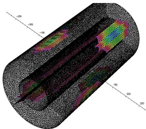
Figure 6: AISHa's hexapole sectors where the field is higher than the coercivity value are shown.
