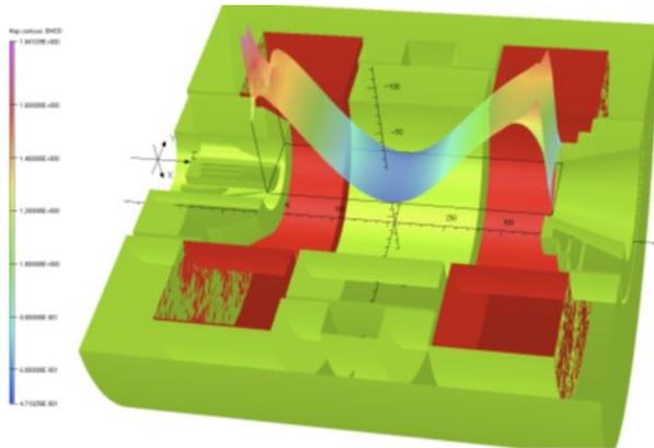
Figure 2: OPERA simulation of the CAESAR axial magnetic field enhancement due to the iron plug insertion.
