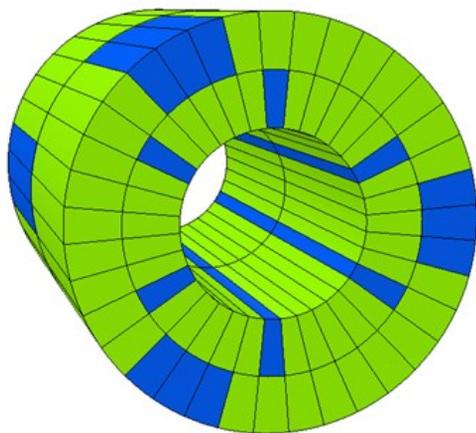
Figure 7: Double shell hexapole geometry (blue sectors have higher coercivity).
