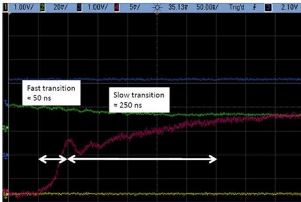
Figure 11: Beam pulse rise time measured.
