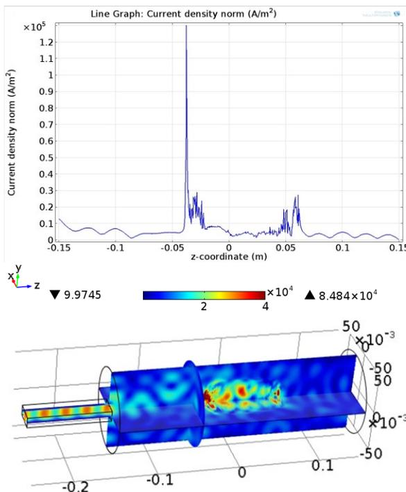
Figure 12: *up* – simulated current density  $j = \bar{\sigma}E$  trend along the plasma chamber axis; *down* – simulated electromagnetic field distribution inside a plasma filled cavity at 8 GHz.
