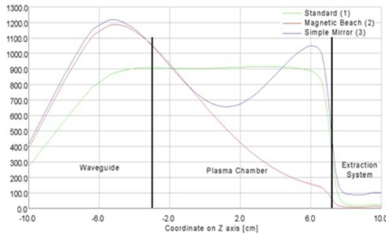
Figure 8: PS-ESS magnetic field profiles.
