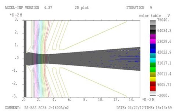
Figure 10: PS-ESS four electrode extraction system.
