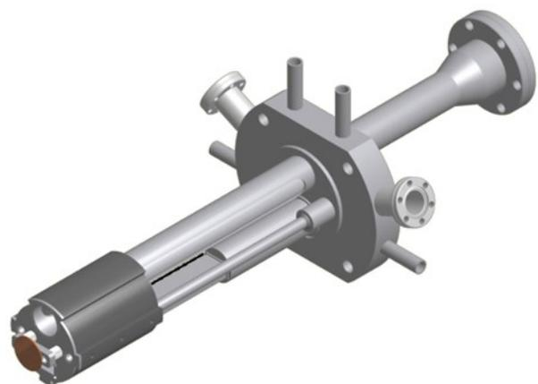
Figure 1: CAESAR new injection system assembly.
