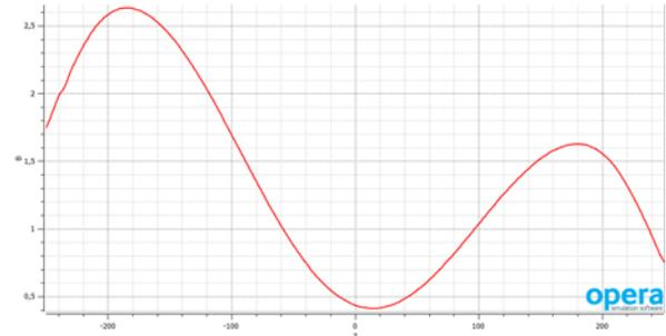
Figure 3: The AISHa magnetic field along plasma chamber axis.
