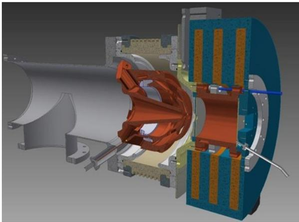
Figure 9: The PS-ESS body source layout.
