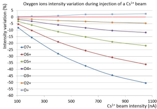
Figure 17: Intensity variation of buffer gas ions when injecting different Cs<sup>+</sup> beam intensities.
