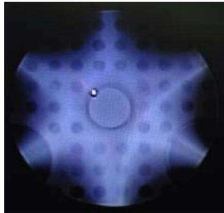
Figure 6: Picture of Argon plasma ignition.
