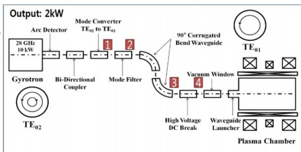
Figure 5: The 28 GHz microwave transmission line from gyrotron to ECR ion source.
