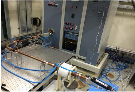
Figure 4: The 28 GHz microwave transmission line from gyrotron to ECR ion source.
