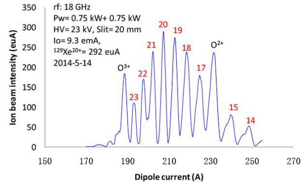
Figure 9: CSD spectrum with the source when optimized on Xe<sup>20+</sup> at 1.5 kW.
