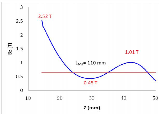
Figure 7: Axial magnetic field distribution when O<sup>6+</sup> optimized.
