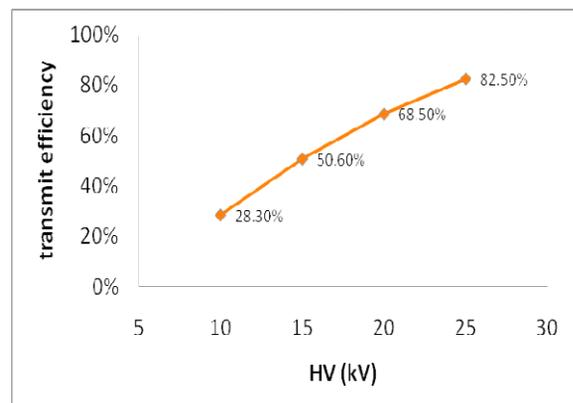
Figure 5: Transmit efficiency of Oxygen beam with different extraction high voltage.
