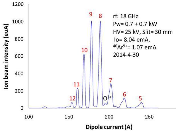
Figure 8: CSD spectrum with the source when optimized on Ar<sup>9+</sup> at 1.4 kW.
