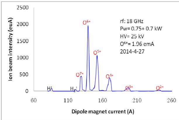
Figure 6: CSD spectrum with the source when optimized on O<sup>6+</sup> at 1.45 kW.
