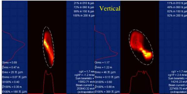
Figure 10: Normalized rms emittances of  $Ar^{8+}$  ion beam extracted from LECR4 ECR ion source.
