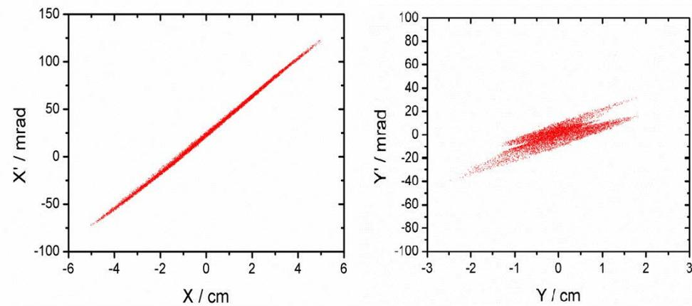
Fig. 3. Simulated phase space distributions of  $C^{5+}$  ion beam by TRACK code
