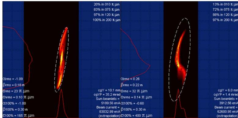
Fig. 2. Measured phase space distributions of  $C^{5+}$  ion beam using  $CH_4$  gas
