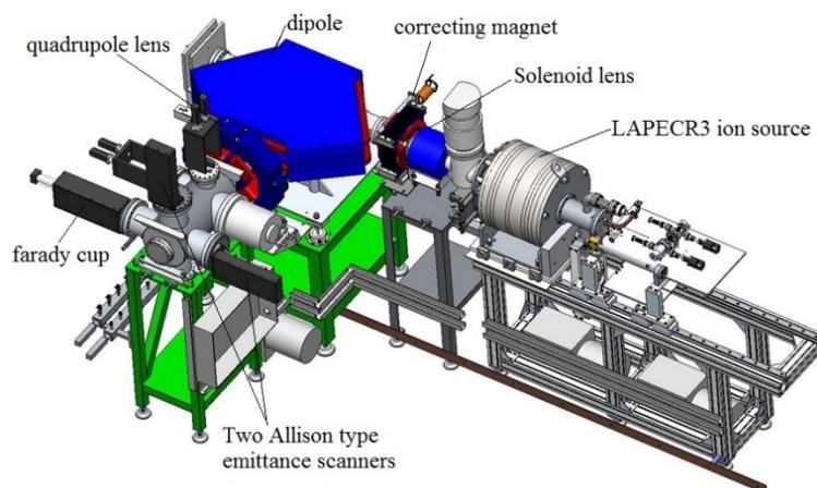
Fig.1. LAPECR3 ion source and the low energy beam line
