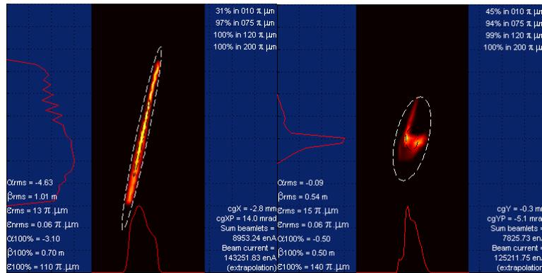
Fig. 4. Measured phase space distributions of  $C^{5+}$  ion beam using  $C_2H_2$  gas
