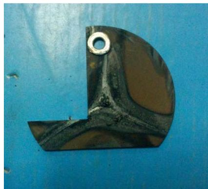
Fig. 6. The photo of the bias voltage plate
