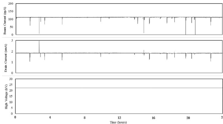
Fig. 5. The curves of the beam current, the drain current and high voltage in 24 hours
