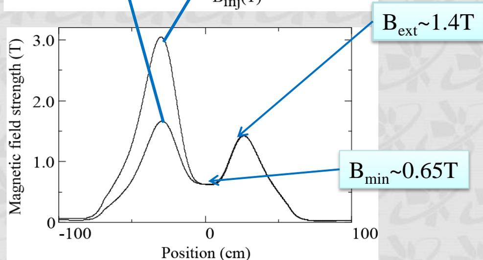
Lower figure shows the magnetic field distribution for investigating the  $B_{inj}$  effect. The  $B_{inj}$  was changed from  $\sim 1.5$  to  $3.1$  T, while keeping the other magnetic field strength ( $B_{ext} \sim 1.45$  T,  $B_{min} \sim 0.65$  T,  $B_r \sim 1.8$  T). Upper figure show the results of rms y-emittance. The emittance **increased from  $\sim 0.09$  to  $\sim 0.17$   $\pi$  mm mrad** with increasing the  $B_{inj}$ .
